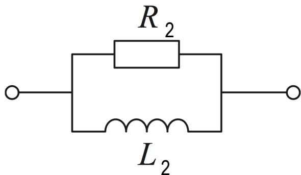
$$\underline{Z} = \frac{R_2 \omega^2 L_2^2 + j\omega L_2 R_2^2}{R_2^2 + \omega^2 L_2^2}$$
