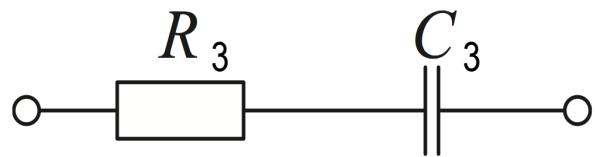
$$\underline{Z} = R_3 + \frac{1}{j\omega C_3} = R_3 - j\frac{1}{\omega C_3}$$
