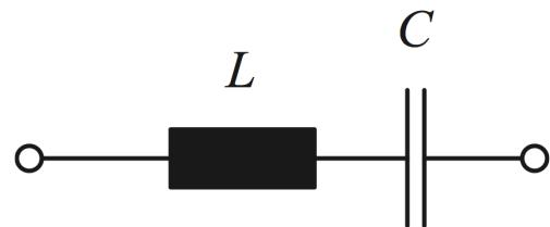
$$Z_{eq} = j\omega L - j\frac{1}{\omega C} = j\frac{\omega^2 LC - 1}{\omega C}$$
