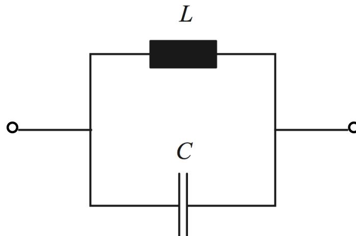
$$Z_{eq} = \frac{1}{\frac{1}{j\omega L} + j\omega C} = \frac{j\omega L}{1 - \omega^2 LC} = j \left( \frac{\omega L}{1 - \omega^2 LC} \right)$$
